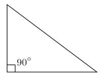
\*The long side opposite the 90° is the hypotenuse. The lengths of all sides can be related through the Pythagorean theorem which states that the sum of the squares of the two non-hypotenuse sides will equal the square of the hypotenuse.
